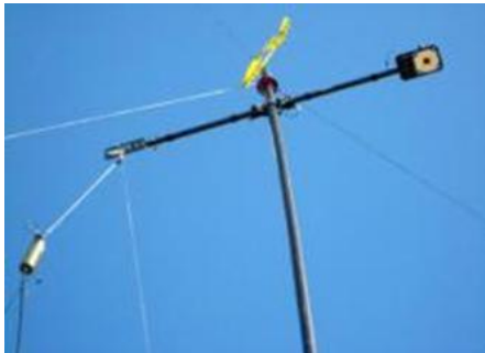
Tactical Sloping-V HF Antenna
