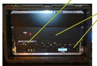
A modified VHSM-5000 modem and associated Pre-Amp (acting as HF Receiver Exciter)
